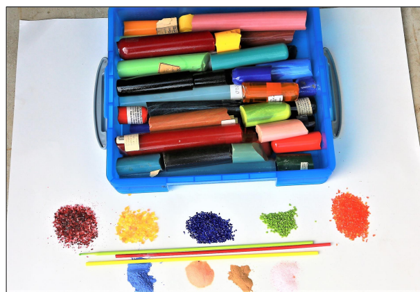
Above is a sample of colored bars and “frit” (powdered glass) that are used by glassblowers to produce hand-made glass items. Note the very thin “straws” that make the colored stripes you find on art glass pieces.
